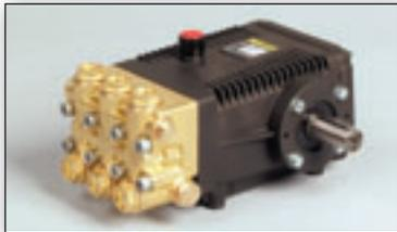
▲ Rugged **High-Pressure Landa Pump**, with three ceramic plungers, forged brass head and 7-year warranty, is connected to the engine by a belt-drive assembly that features cast-iron bushing **Pulleys** and two notched "V" cogged belts, which provide a cooler operation and longer life; also **Two-Bolt Adjustment** makes it easy to adjust the belt tension.
